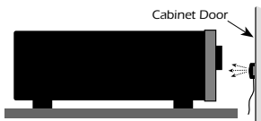
Fig. 5b IRE-2.0 attached to inside of cabinet door directly opposite IR sensor window
